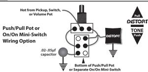
NOTE: When the push/pull pot is pulled up Black Ice Distort is activated. Clockwise rotation will increase distortion. When pot is pushed down, tone control operates normally.
