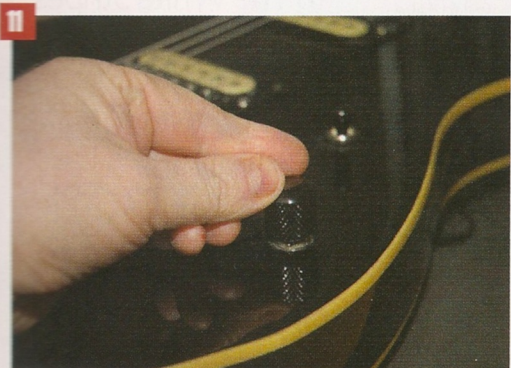
8 If your guitar has a push/pull tone control, you can wire it so that when its knob is up, the Black Ice is activated. Push the knob down, and the tone circuit kicks back in.
